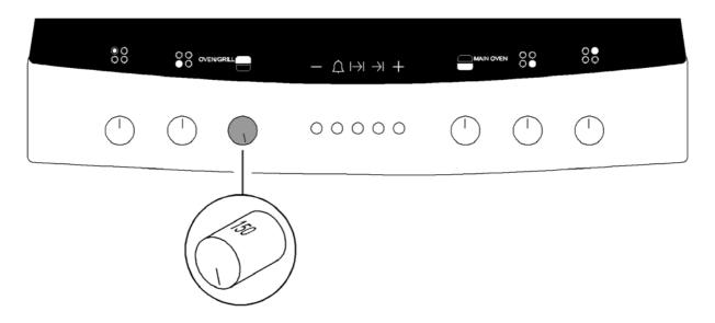
Turn the top oven temperature control to the required setting. Our diagram shows the oven set to 150°C. Close the oven door.
